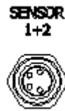
Fig. 6-11: Sensor socket (M8 4-pole) at the back side of the control system
