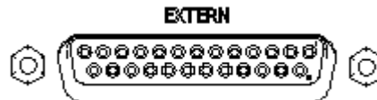
Fig. 6-13: Extern socket (Sub-D 25-pole) at the back side of the control system
